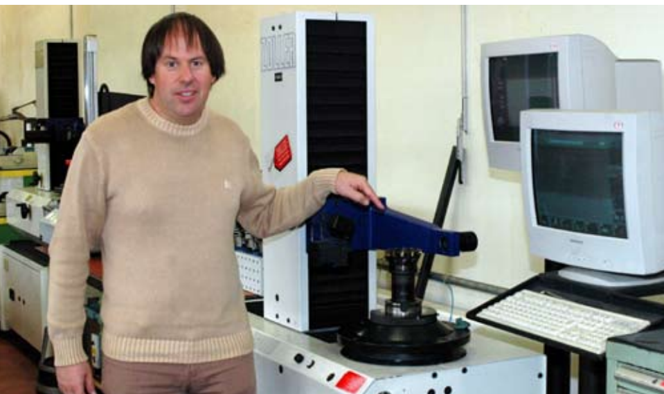
Tornos' Pierre-Yves Gurtner at a presetting device: "Thanks to TDM we have achieved here an automated process, with flexibility, accuracy, and a high level of tool availability."
