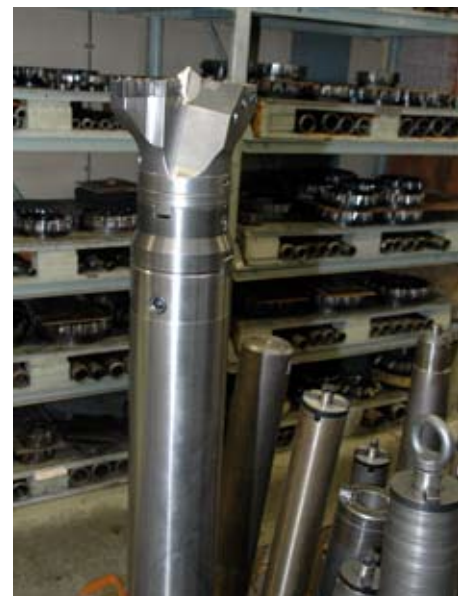
Long overhanging tools like stands, pestles and headpieces are often required to make large-scale parts for presses. The interface between TDM and AutoCAD is indispensable during assembly in the tool presetting area.
