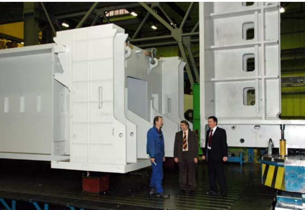
In Erfurt, stands weighing up to 5 metric tons fall under „small parts manufacturing“! Headpieces and tables may weigh up to 200 metric tons.
