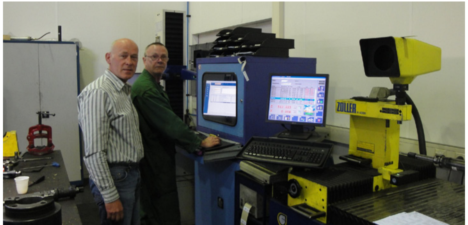
TDM Project Director Ton Heurnink (at left) standing with tool presetter Derk Moll at the Zoller presetting device. Tool data management is integrated by means of a standard interface: target data and measurement program parameters are relayed automatically to the setting system, and actual values are relayed back again.
