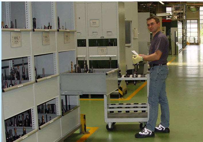
With TDMshopcontrol, Mr Schneier has no difficulty in managing 3 set-ups a day, each with 50 to 80 tools for 10 machining centers. (Photo: Mr. Schneier with tool trolley at the stand by magazine)
