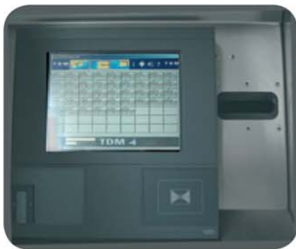
Indexable insert ejection via touchscreen: TDM's new TDMstoreasy software at Liebherr controls loading and dispensing at a vending machine from Sandvik. The team member in the production facilities inserts his plant data acquisition card in the slot at the right, uses the touchscreen to select the required indexable inserts, and these are then dispensed automatically
