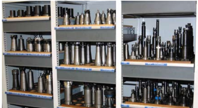
There is no lack of tools at MTU. The TDM software system keeps track of 42,000 single tools, 21,000 tool assemblies, and 28,000 NC tool lists.
