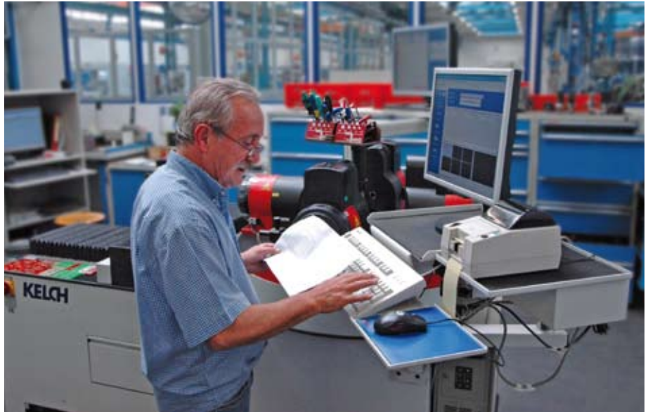
A typical presetting station in the production area. At Schütte Company in Cologne, Germany, TDM software automatically delivers tool data to the Kelch presetting device.
