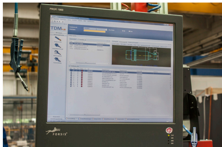
The TDM-order shows the list of items and a drawing of the tool assembly which has to be put together.
