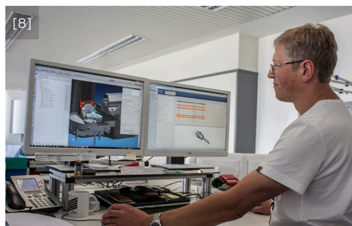
[8] CAD/CAM programming: Sample tool (inner torsion bar) and sample part for the transfer of turning tools from TDM (right screen) to NX (left screen).
