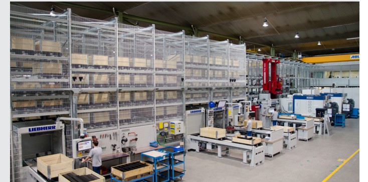
The high-bay stacking storage system, in which the components are temporarily stored on carrier plates until they are needed for machining and also automatically removed when required.
