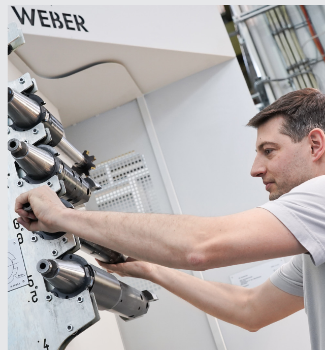
Inserting the tool assemblies into the loading/unloading station.
