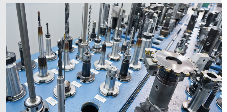
Unique tool identification via barcode.
