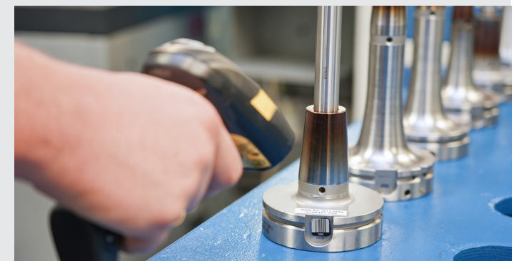
Unique tool identification via barcode.
